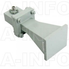
LB-90-10-C-SFSPO Standard Gain Horn Antenna 8.2-12.4GHz 10dB Gain SMA Female
