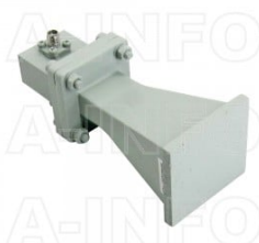
LB-90-10-C-3.5FSPO Standard Gain Horn Antenna 8.2-12.4GHz 10dB Gain 3.5mm Female
