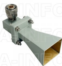
LB-90-10-C-7 Standard Gain Horn Antenna 8.2-12.4GHz 10dB Gain 7mm
